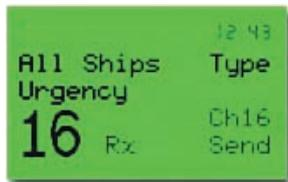
Any vessel that may require urgent assistance, but where life is not in immediate danger, can initiate an all ships urgency call. The vessel may be drifting without power or lost steering, and requires assistance to be towed to safety.
