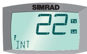
IN ADDITION TO SHOWING THE CHANNEL IN USE, BATTERY CONDITION AND OPERATION STATUS IS DISPLAYED.
