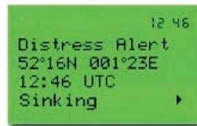
In an emergency situation the DSC radios have dedicated distress functions that can be directly activated with the distress button.
